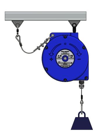
\*- SECONDARY SUPPORT CABLE SHOULD BE AS SHORT AS POSSIBLE, ALLOWING RETRACTOR TO DROP NO MORE THAN 6 TO 12 INCHES [150-300 mm] IF THE PRIMARY CONNECTION IS RELEASED.
